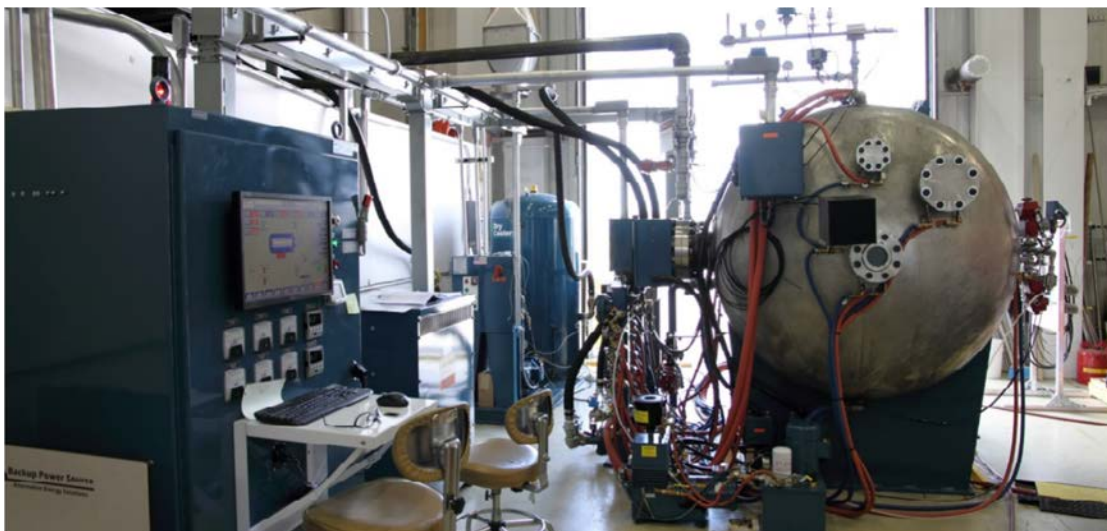
Figure 18. SPECTR test facility used for high-pressure and high-temperature testing of components as well as cyclic testing.
