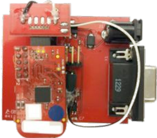
Figure 8. ZigBee coordinator implementation
