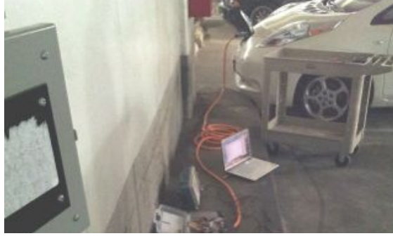
Fig. 15: Experiment setup of changing pilot signal
