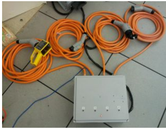
Fig. 4: Realization of 4 channel charging station
