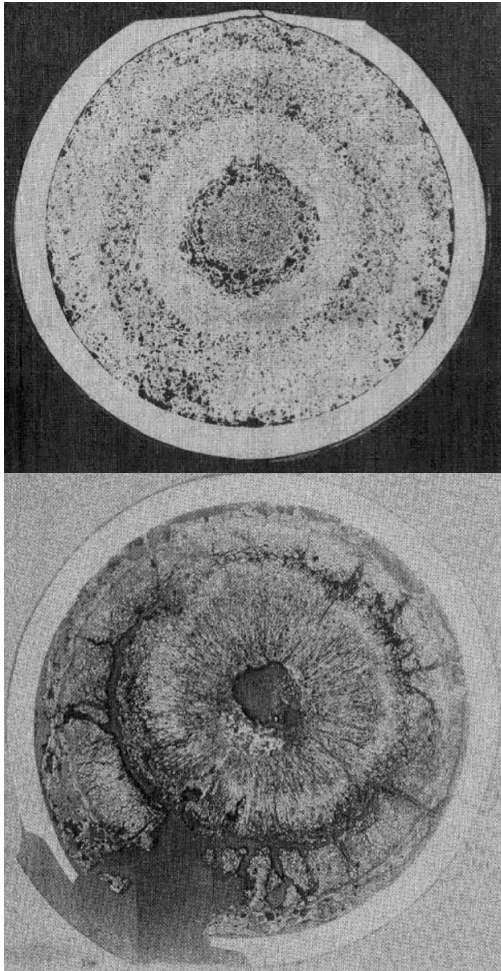
Fig. 6. Comparison of breach in cladding for metal fuel (top) 18 and oxide fuel (bottom) 19 .
