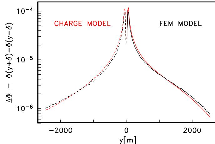
**(right)** eyeball-minimized data misfit of time lapse inline potential differences.  $\lambda = 5.6\text{E-}15$  C/m,  $q = 1.7\text{E-}11$  C.
