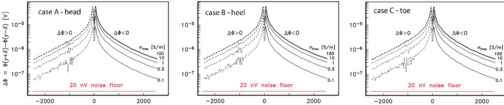
Inline scattered potential differences ( $\delta = 50$  m) as a function of fracture conductivity over the range 0.1–100 S/m for a -1 A source at  $y = -1000$  m and +1 A source located at either the well head, heel, or toe (cases A-C). Dashed lines indicate negative values; solid lines, positive.
