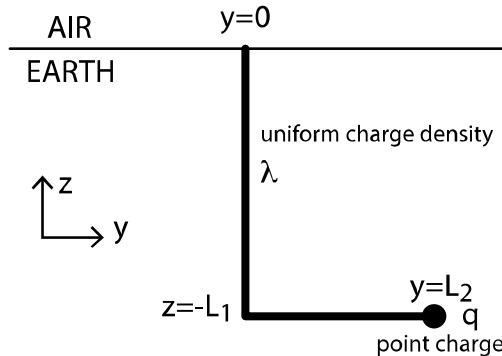
**(left)** problem setup for LQS inversion of toe-fracture data with known fracture location,  $s$ . Inversion is linear in charge magnitudes  $\lambda$  and  $q$ .
