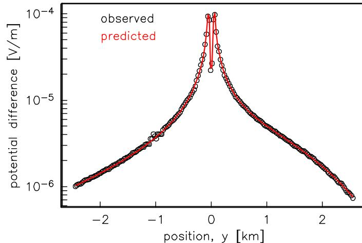
**(right)** L2-minimized data misfit of time lapse inline potential differences.  $\lambda = 5.1\text{E-}15$  C/m,  $q = 1.8\text{E-}11$  C.
