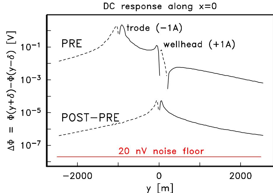
Potential differences computed using  $100$  m electrode separation,  $\delta = 50$  m. For reference, also shown is the  $20$  nV noise floor for the 32-bit ZEN receiver from Zonge Engineering (<http://zonge.com/instruments-home/systems/distributed-em-systems/>).
