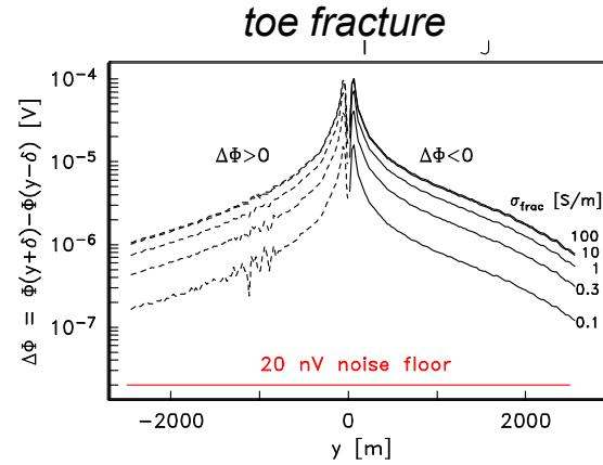
Inline scattered potential differences ( $\delta = 50$  m) as a function of fracture conductivity over the range 0.1–100 S/m for a  $-1$  A source at  $y = -1000$  m and  $+1$  A source, fractures located at either the well heel (**left**), or toe (**right**). Dashed lines indicate negative values; solid lines, positive.
