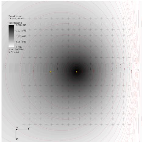
**(above)** Broaden the array to a *massive* 20x20 grid of 2-component measurements on a 4x4 km area. Time-lapse potentials in grey scale with red contours. Stations indicated by + signs. Well head and ground point indicated by yellow dots.
