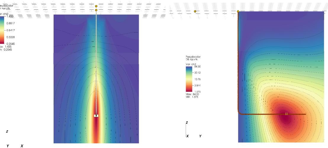
Color scaled L2 norm values of optimal  $(\lambda, q)$  pairs for candidate 's' points in a plane orthogonal to the horizontal section of the well bore and through the fracture set (**left**), and in a plane containing the entire well bore (**right**).
