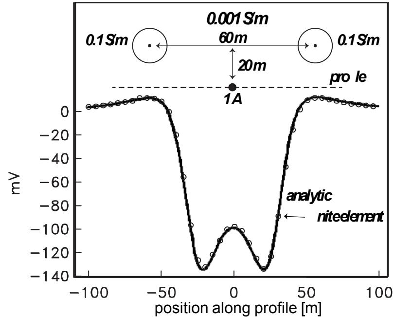
*(above)* comparison of finite element and analytic solutions of scattered electric potential for an offset point source
