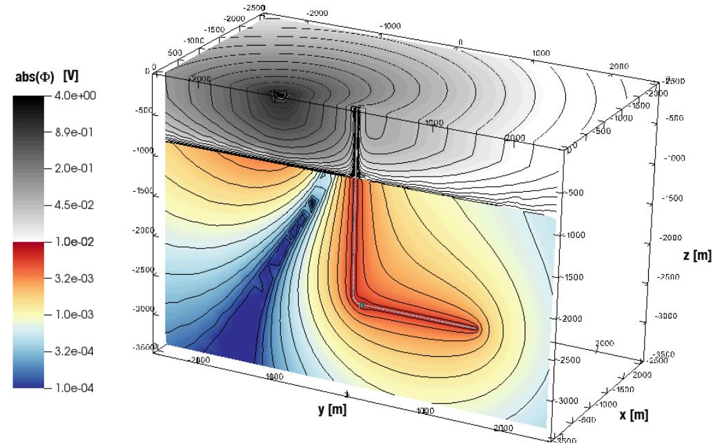
Generally small amplitudes of the potential in the region below  $z = -800$  m are consistent with its relatively high  $0.03$  S/m conductivity – in contrast to the low ( $< 0.001$  S/m) conductivity in the region above  $z = -800$  m.
