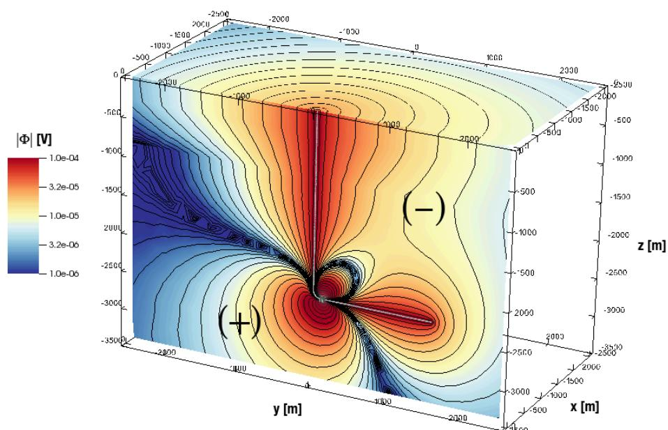
**Empirical LQS inversion:** invert time-lapse surface data for linear charge density ( $\lambda$ ) on the well casing; point charge  $q$  at the fracture, and position  $s$  of the fracture.
