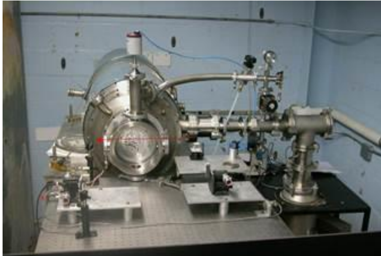
Figure 2. A picture of the accelerator used for direct electron beam injection into gas experiments. The red line shows the HeNe laser used to obtain line-integrated electron measurements.
