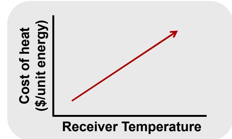
However, higher T allows **more efficient** production of electricity or H<sub>2</sub>
