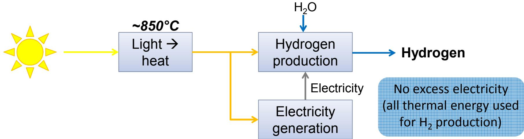
For Case 2, **9%** of thermal energy is used directly for  $\text{H}_2$  production, **91%** of thermal energy is used for electricity generation
