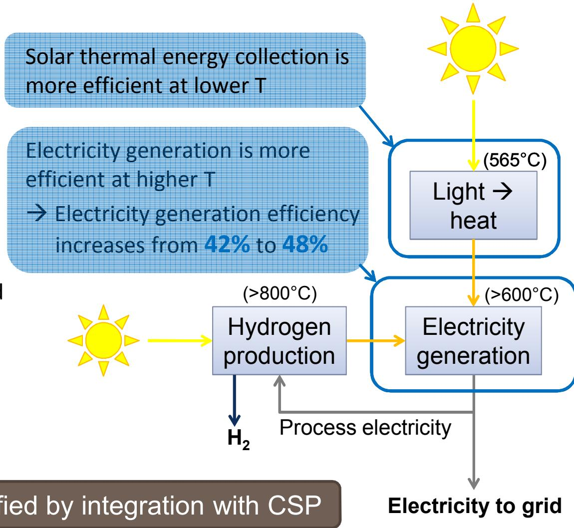
Value of waste heat is amplified by integration with CSP
