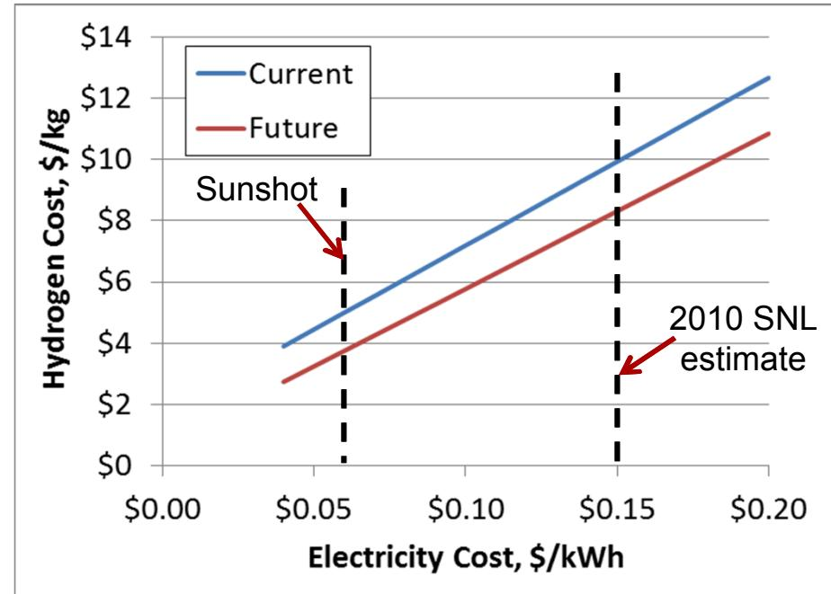
Results from H2A model of Hydrogen Production from PEM Electrolysis .
