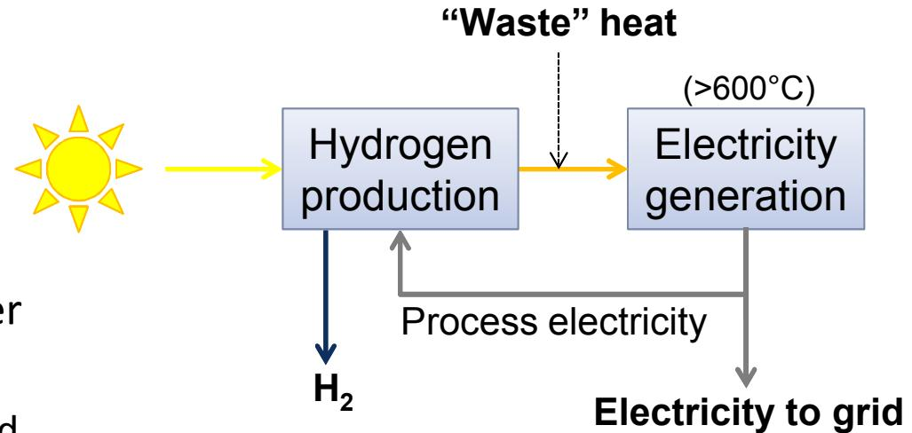
No need to purchase grid electricity, but smaller scale of power generation reduces efficiency and increases cost compared to full-scale CSP
