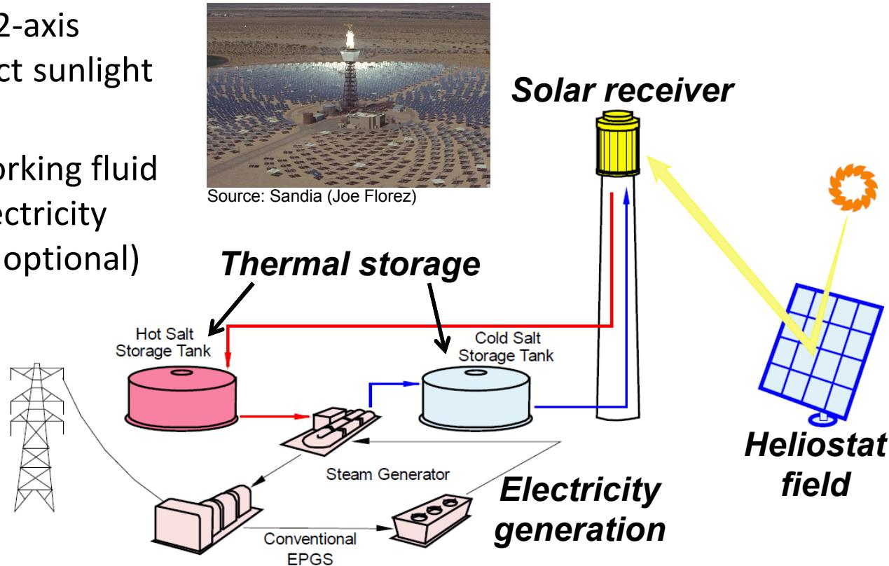
Baseline CSP plant: Power Tower configuration with molten salt thermal storage and subcritical Rankine cycle electricity generation
