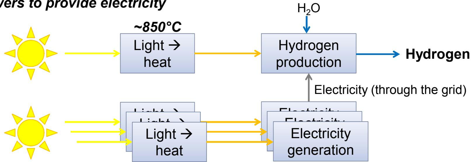
**11 additional CSP towers** would be necessary to supply necessary electricity for each tower supplying exclusively heat for  $H_2$  production
