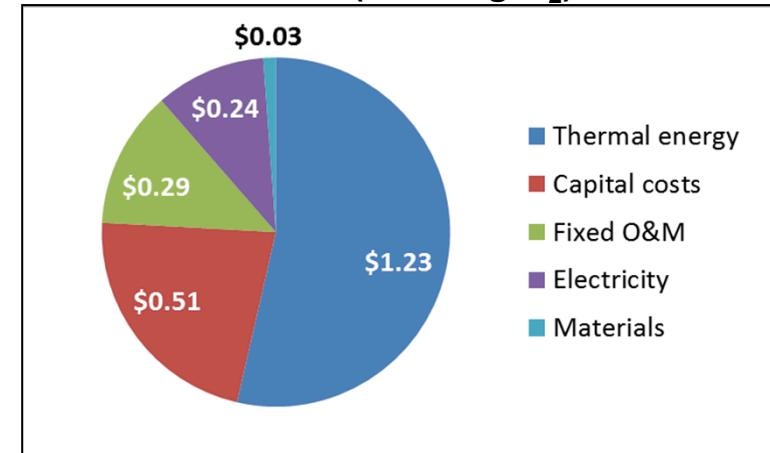
Source: “Ultimate” Central Hydrogen Production from Solar Thermo-Chemical Cycle, H2A Case Study
