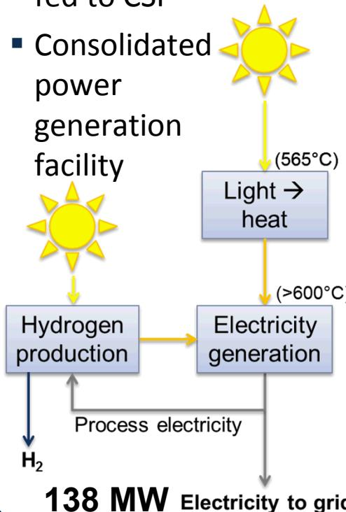
Electricity generation efficiency increases from **42%** to **48%** at higher T
