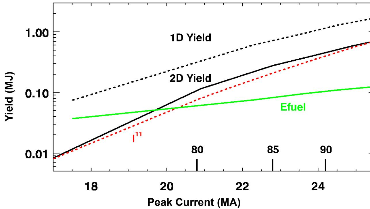
Capsule parameters (radius, fuel density, fuel preheat, and  $B_z$ ) are optimized at each value of the drive current.
