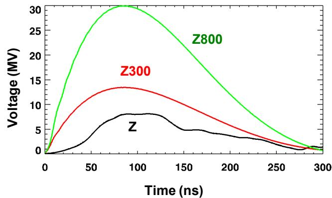
Present experiments on Z at 18 MA do not have optimal values of preheat or applied field according to simulation
