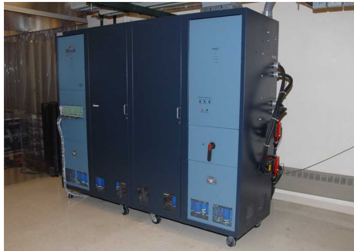
72V 1000A Bitrode (2 Channels)
