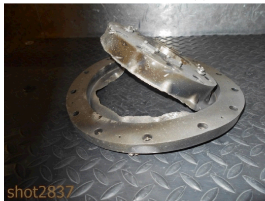
Top anode plate damage indicates severity of loss
