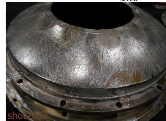
Metal spray coats middle anode plate
