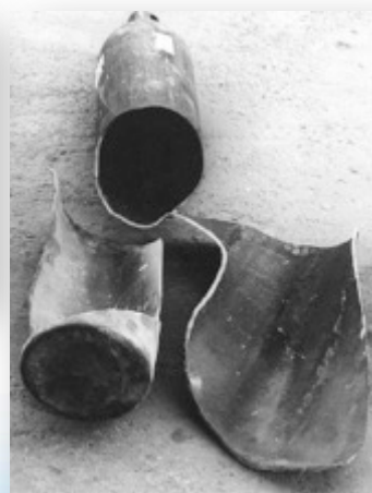
example of embrittlement failure from the 1970's
