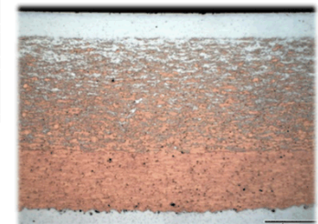
Cu-Al plasma sprayed graded density coating
