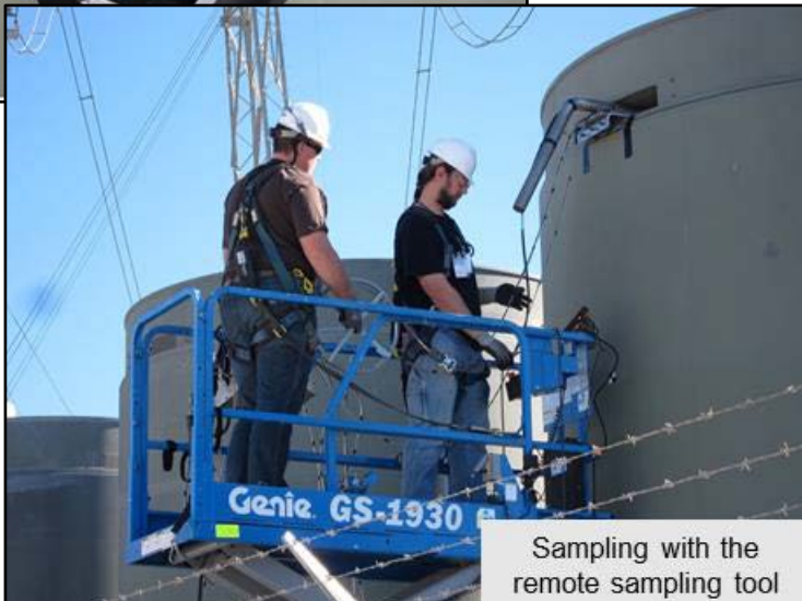
Sampling a HI-STORM 100 canister at Diablo Canyon
