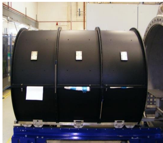
Figure 61. Compact product block design (3 blocks shown) able to accommodate 6 versus 5 strips
