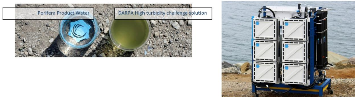
Figure 6. Porifera Treated Water (left) and Pilot System (right) [7]
