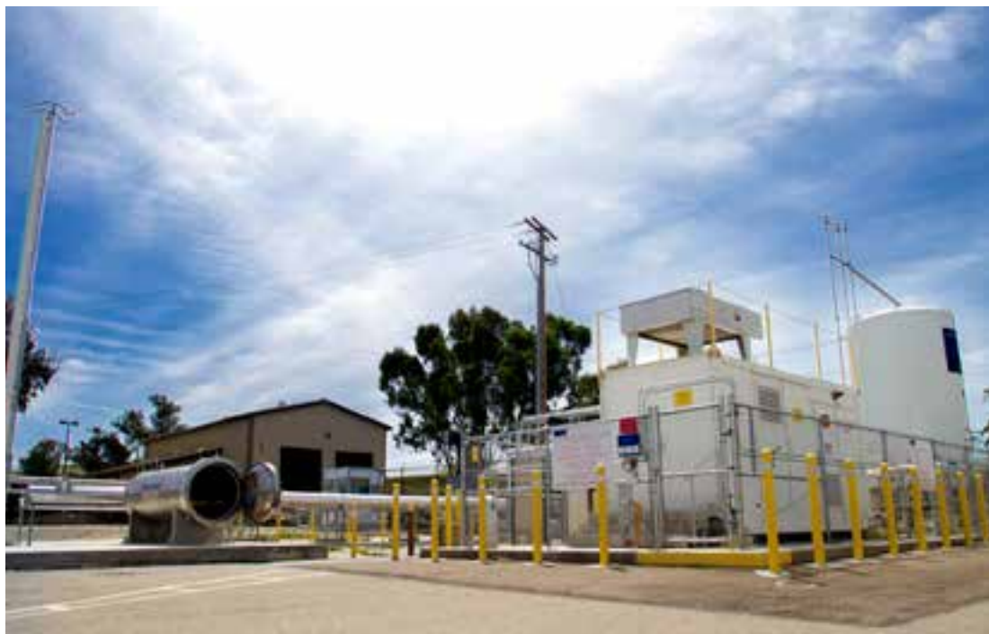
The two main components of Lawrence Livermore's Cryogenic Hydrogen Test Facility are (left) the stainless steel containment unit used to test prototype hydrogen storage vessels and (right) the liquid-hydrogen pump built by Munich-based Linde Corporation.
