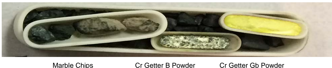
Figure 2-94. Cr Getter Materials Tested for 1000 Hours at 800°C in Dry Air over Cr Pieces
