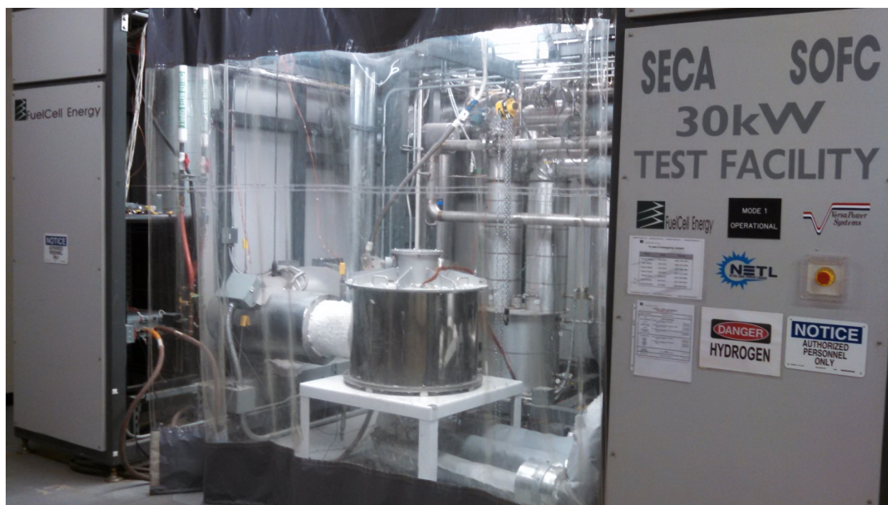
Figure 2-133. 3 kW Thermally Self-sustaining SOFC Stack Module Installed in FCE Danbury Test Facility TF-30kW-5
