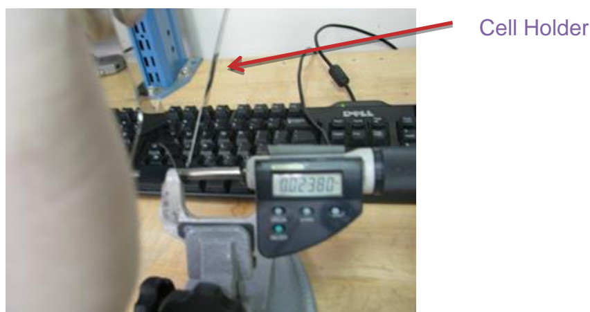
Figure 2-45. Cell Holder Thickness Measurement Using Micrometer Caliper
