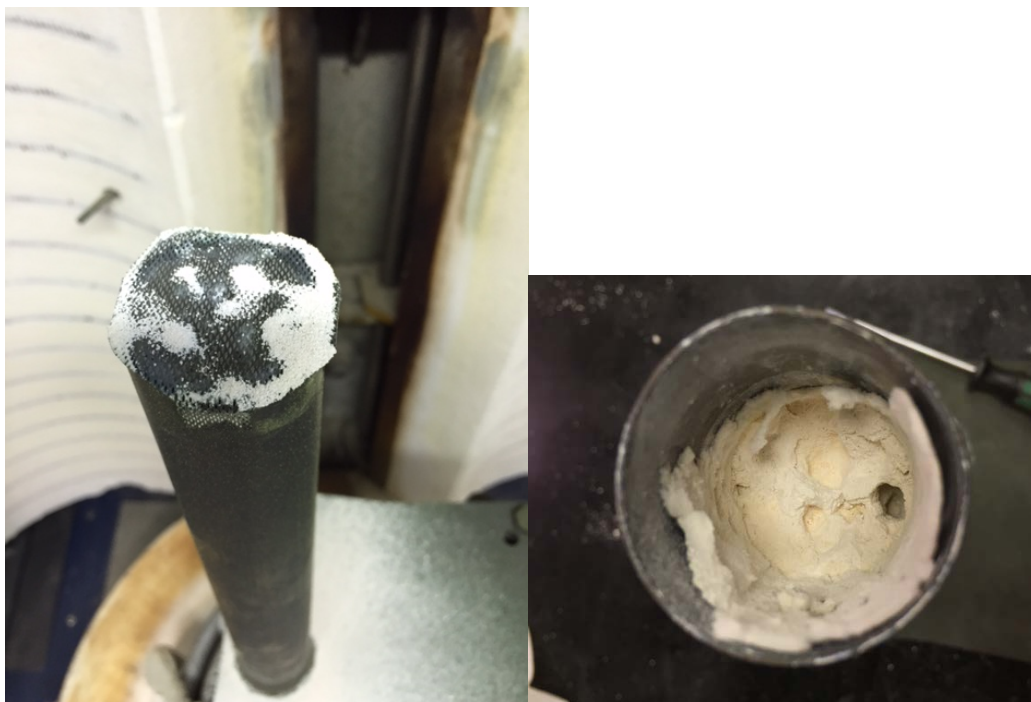
Figure 2-93. Proof of Concept Cr-Getter Filter Test #2 – Post-Test
