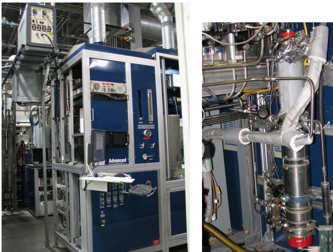
Figure 2-131. Test Stand Cathode Gas Humidifier Upgrade (left) with In-Stand Dew-Point Humidifier Vessel (right)
