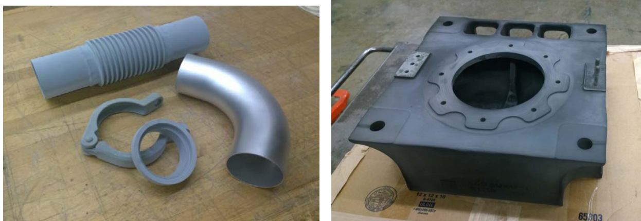
Figure 3-2. Aluminized Non-Repeat Module Components. Left- Al Coated Ducts (Prior to Heat treatment). Right- Cast Compression Plate (After Heat Treatment).
