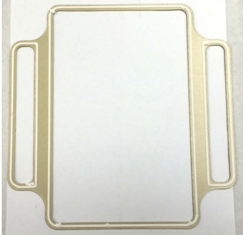
Figure 2-88. Dispensing Trials on Thermicullite Seal to Verify the Process
