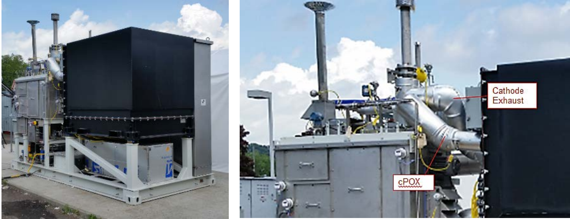
Figure 5-24 Fabrication Photos – Module and BoP (left), Instrumentation Rack & Electrical Panel (right)
