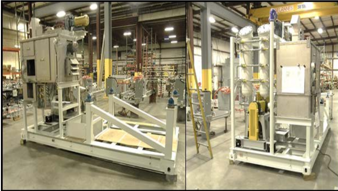
Figure 5-19 Fabrication Photos – Structural Skid w/ Desiccant and Desulfurizer
