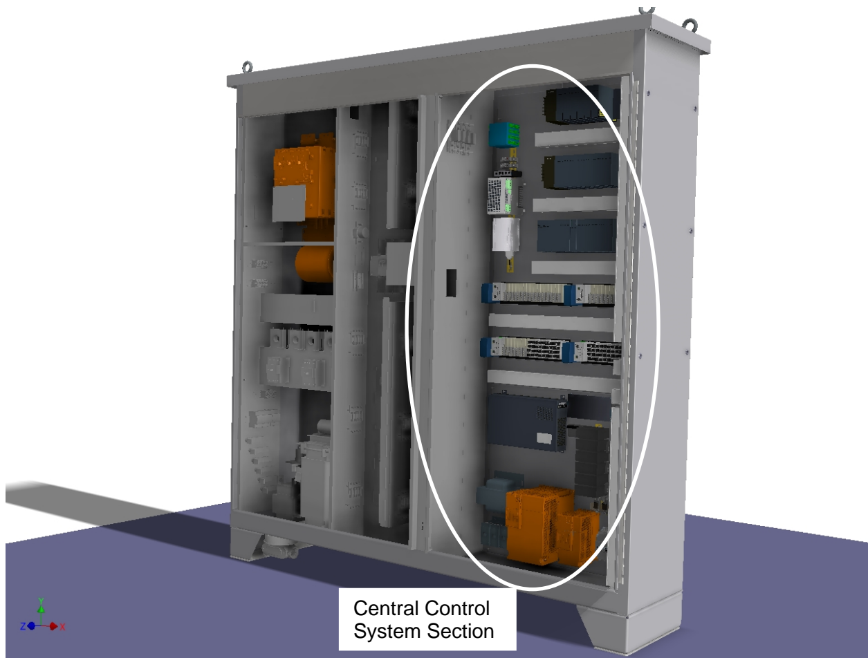
Figure 5-18. EBOP Enclosure Showing Central Control System Section.
