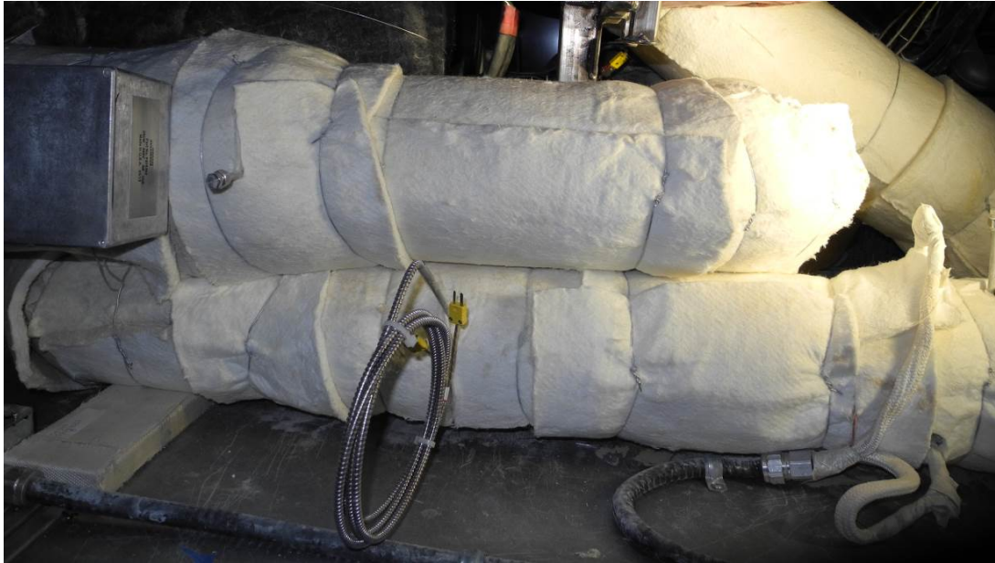
Figure 2-132. Newly Installed Cathode and Anode Preheaters after Insulation Work in Test Stand #28
