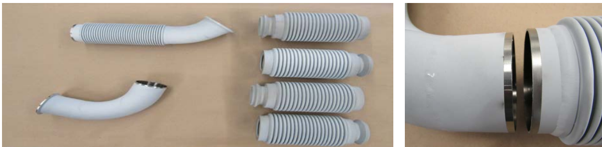
Figure 3-5. (left) Piping Components Aluminized (right) Piping Components Masked and Aluminized
