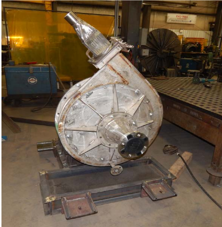
Figure 5-7. Photograph of Anode Recycle Blower at Vendor's Shop, Prior to Painting of the Base
