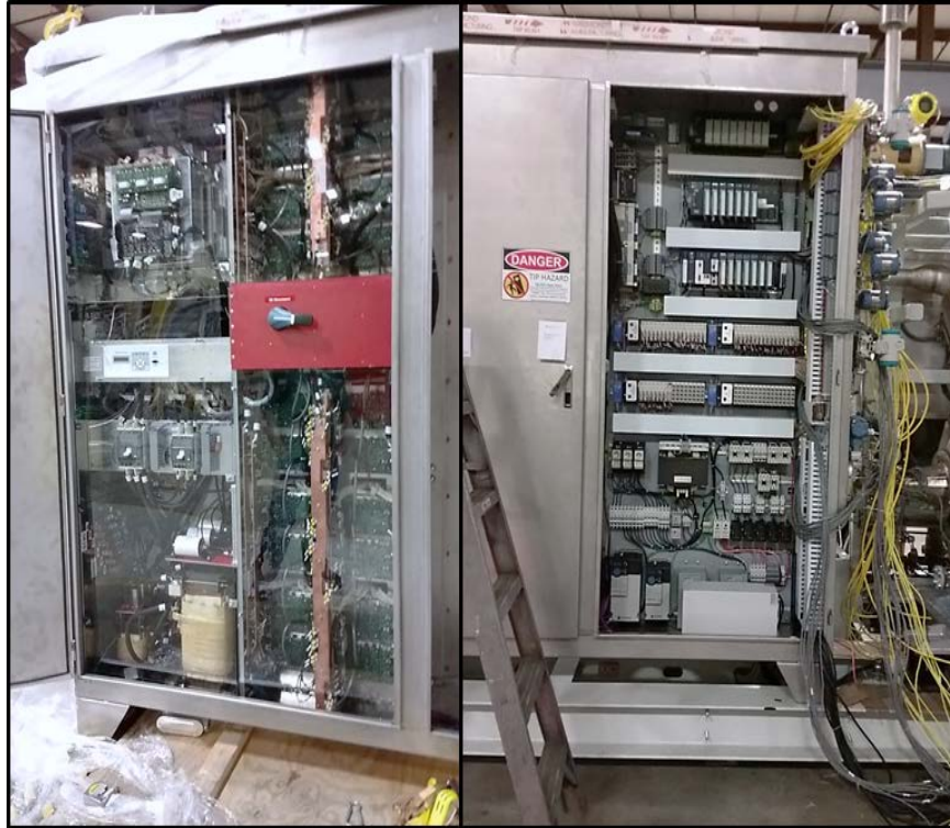
Figure 5-21 Fabrication Photos – Inverter & Control Sides of EBOP Cabinet
