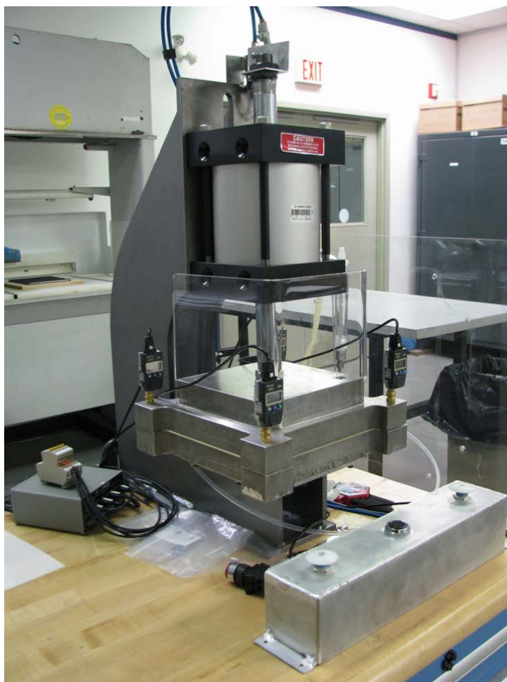
Figure 2-53. Cell Leak, Thickness, and Flatness Checker
