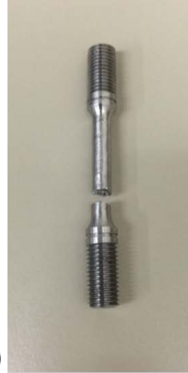
Figure 24 Tensile test of the ferritic steel #2 after solutionization at 1200 °C for 8 h and aging at 600 °C for 12 h.
