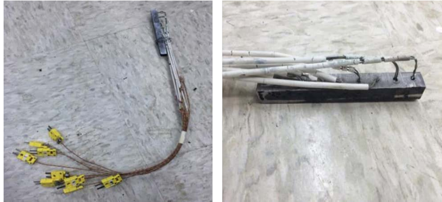
Figure 6 Sample for a gradient temperature precipitation heat treatment. Nine holes drilled on a steel bar with 0.5-inch spacing. Nine individual type-K thermocouples were attached to the sample and bent towards one direction for attachment to the temperature measurement unit.
