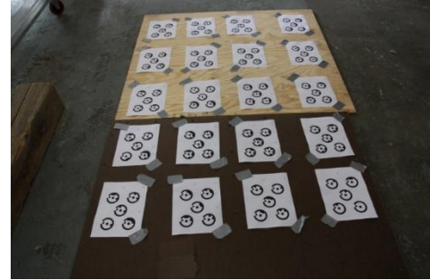
Figure 28 – Photogrammetry targets on floor and sheet of plywood, used for initial camera calibration.
