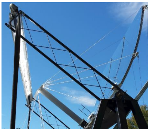
Figure 7 - Optical prototype receiver and collector assembly during an on-sun test.
