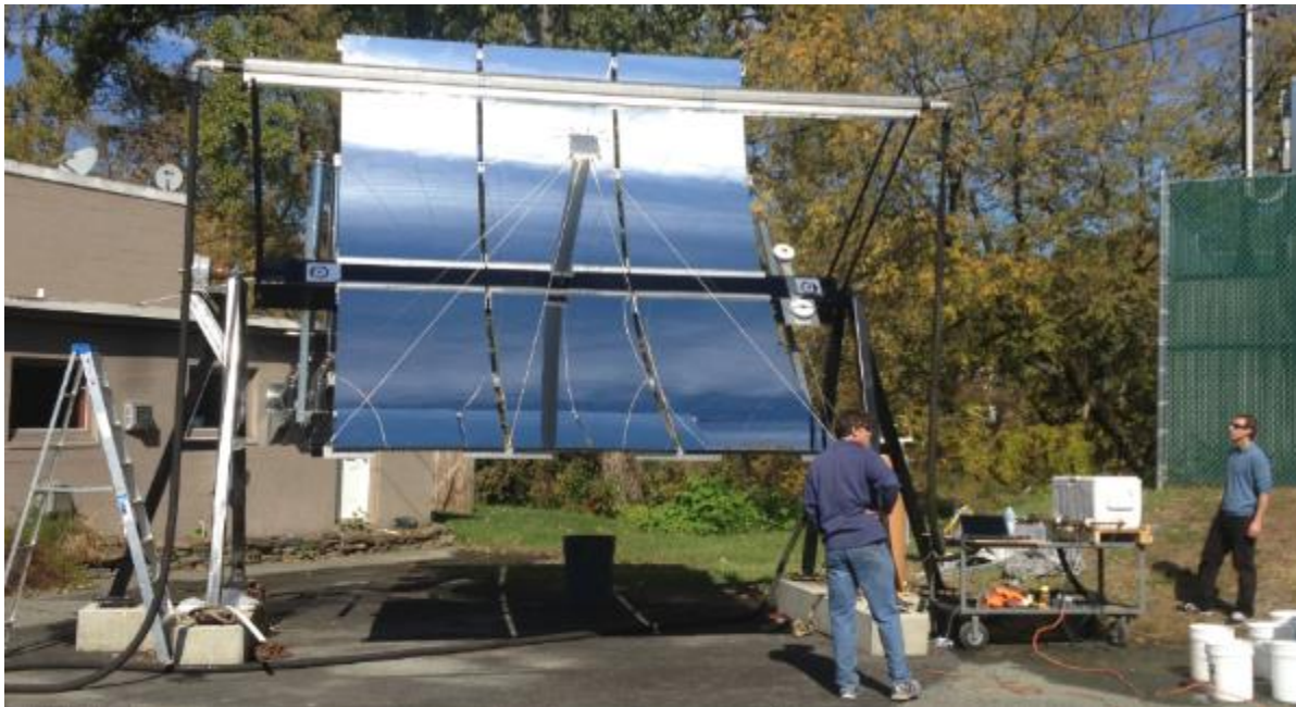
Figure 14 – Optical efficiency test in operation. Test cart is shown at lower right; pyranometers are visible on right side of mirror.
