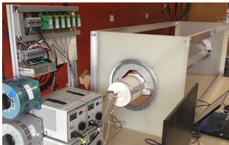
Figure 8 – NT heat loss test stand during test. Receiver is mounted in rotating frame on lazy-susan bearings to facilitate testing over a range of tilt angles.
