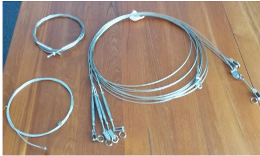
Figure 22 – Suspension cables. Clockwise from lower left: swaged Solaflect cable for suspension heliostat, stud-terminated stainless cable for railings, and cables for prototype suspension trough. Custom cable systems are readily available from railing and marine vendors.
