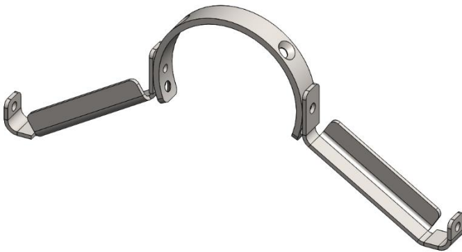
Figure 5— Absorber tube support bracket assembly for thermal test prototype. Collar is cut from tubing stock, while arms are bent sheet metal. Four spacers (ceramic in heat loss prototype, PTFE in optical prototype) on screws such that tube is supported but can slide axially during heating and cooling cycles. Brackets act to stiffen shell, which in turn supports absorber tube. With a bracket every ~2 m, absorber tube deflections are reduced.
