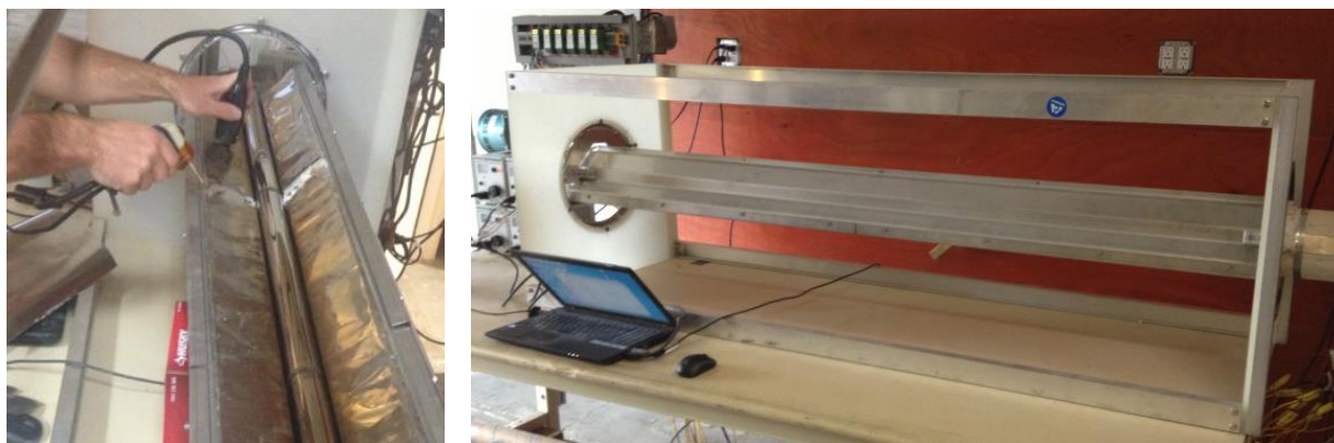
Figure 6– (Left) Assembly of thermal test receiver, spot-welding foil to enclose insulation. Tube in image is coated with an IR reflector layer. (Right) Assembled receiver in rotating frame for testing.
