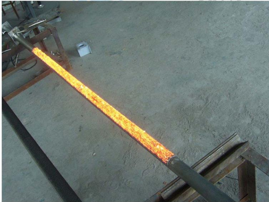
Figure 11 – Gas-Fired Pipe Burner
