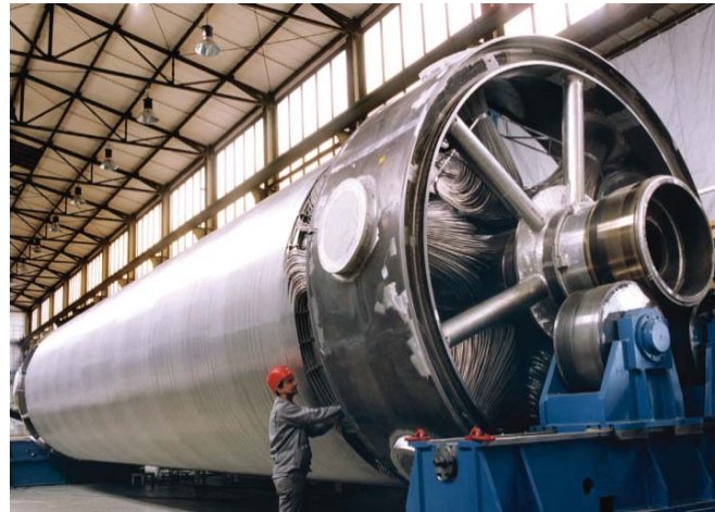
Linde Gas Coil-Wound \beta from 10 to 300 [m 2 /m 3 ]
