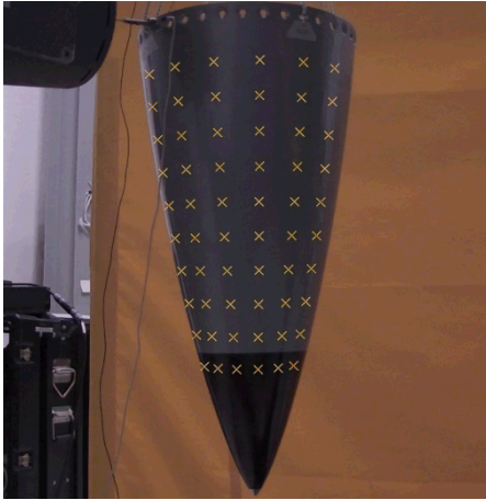
Figure 8: Laser camera view showing measurement points for one scan.
