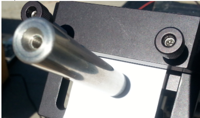
Fig. 23: Detailed illustration of the aligning rod with shadow
