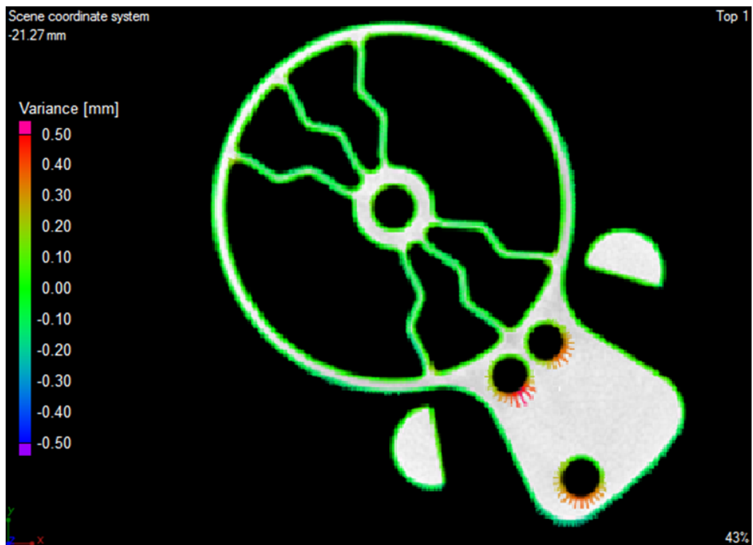
Figure 18: CT Scan Cross Sections of the NSC SLS built part
