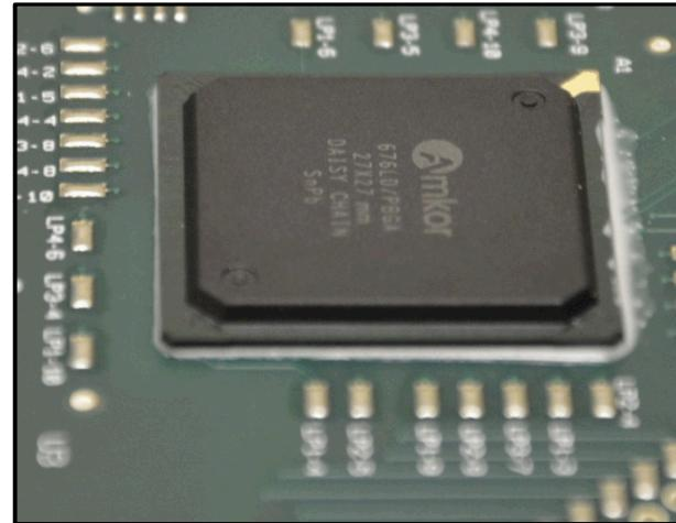
After a PBGA (or other surface mount component) is attached to a circuit board, an adhesive underfill is often applied to improve lifetime performance
