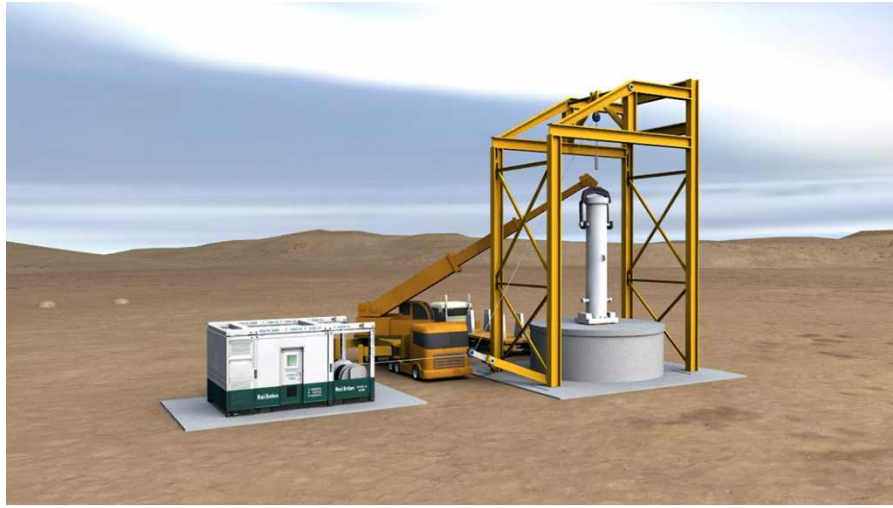
Figure 6 wireline handling and emplacement components.
