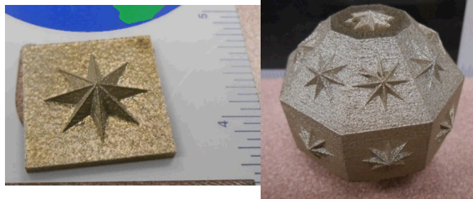
Siemens star geometries for resolution evaluation
