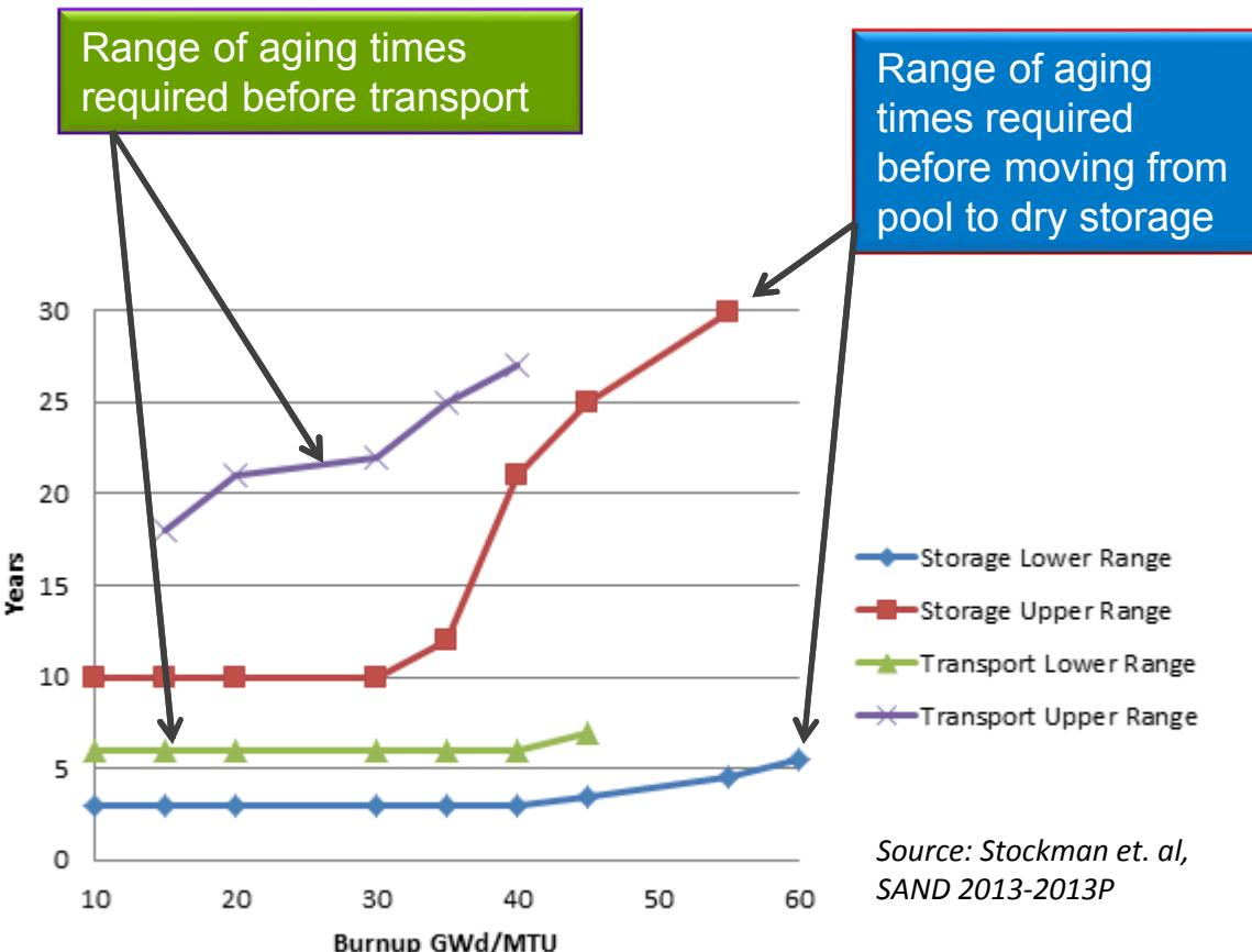
Minimum cooling times for multiple cask/canister systems, based on NRC certificates of compliance for specific designs. Variation in times is due to the diversity of the current inventory, dominated by DPC size and heat transfer capabilities.
