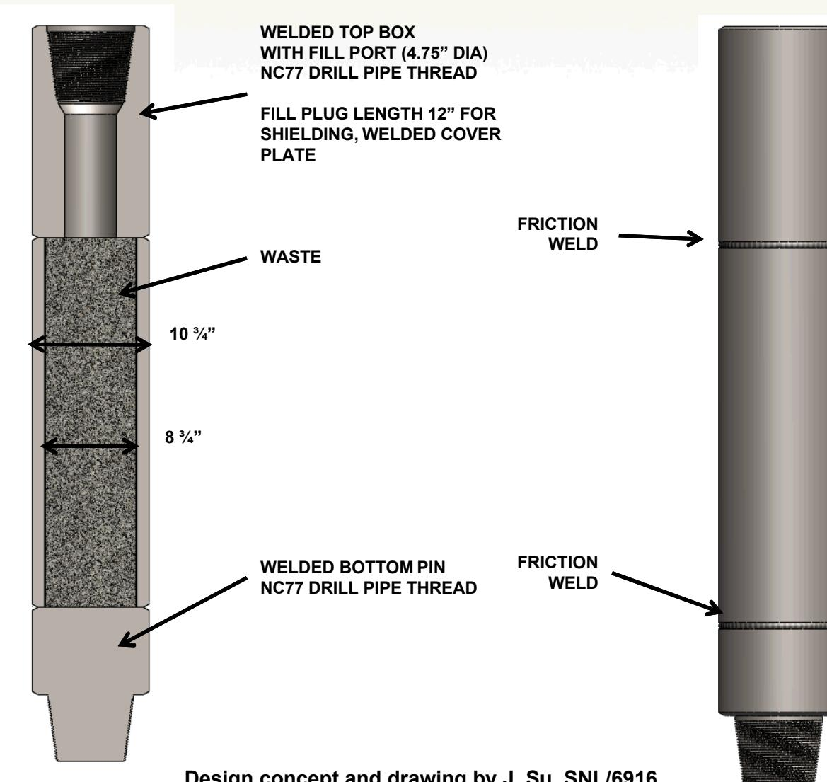
All weld heat mitigation except cover plate, done before waste loading.
