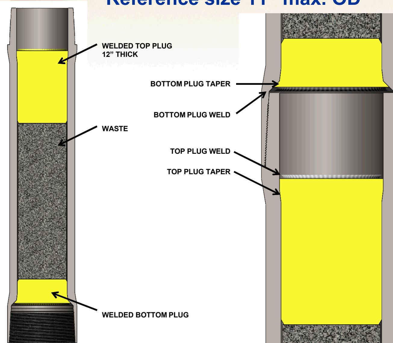
Internal-flush design for canistered waste forms.
