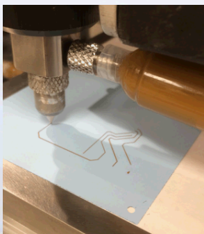
DW circuit fabrication
