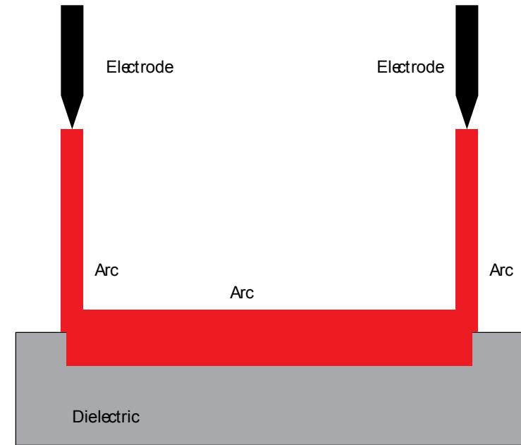
Early times: Air breakdown with the dielectric acting like a metal
