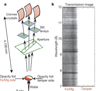
Figure 1 | Experiment diagram and example transmission image. a. Three to four spectrometers view the 'half-moon'-shaped tamped iron/magnesium sample (not to scale). Each uses multiple slits to project spatially resolved images onto a convex crystal that disperses the spectrum before recording on film (not shown). The inset shows the uncorrected transmission image.
