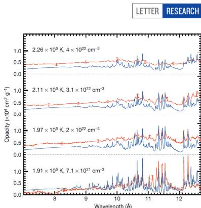
Figure 2 | Measured iron opacity spectra at four  $T_e/n_e$  values compared with calculations. The SCRAM<sup>TM</sup> model calculations (blue lines) account for the instrument resolution. Red lines denote the measurements and the error bars
