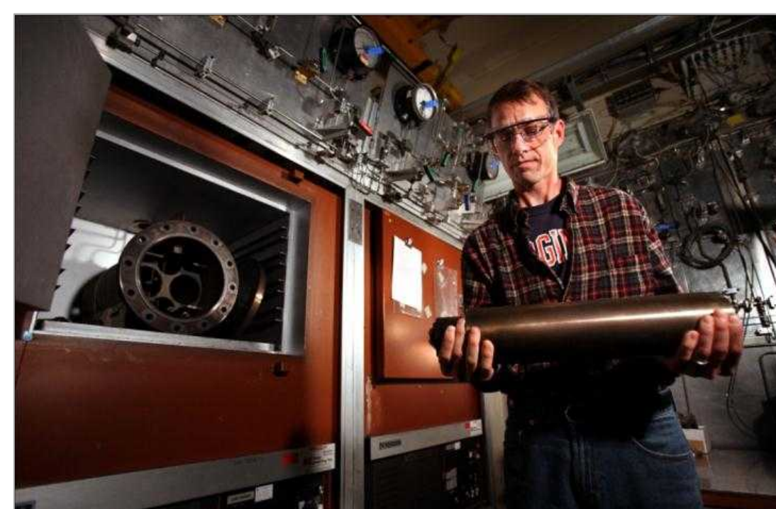
Hydrogen pre-charging: 300°C, 20,000psi, 16 days, resulting in a minimum of 0.8 at% H
