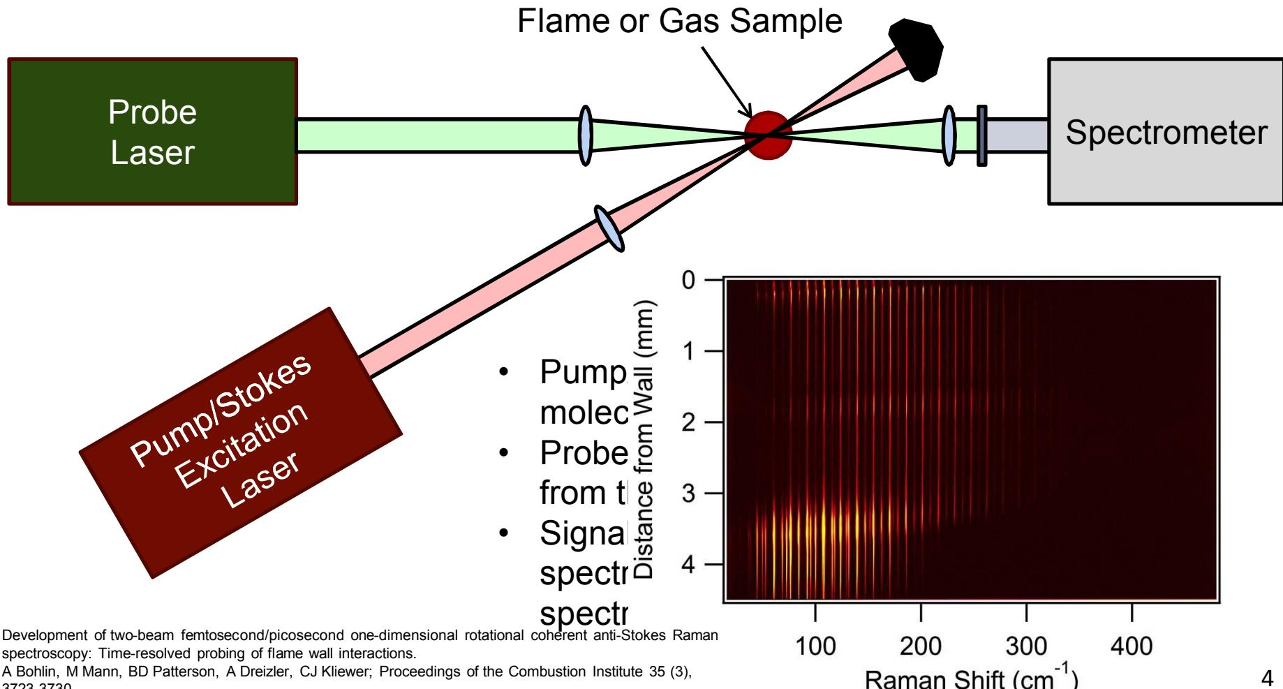
Development of two-beam femtosecond/picosecond one-dimensional rotational coherent anti-Stokes Raman spectroscopy: Time-resolved probing of flame wall interactions.
