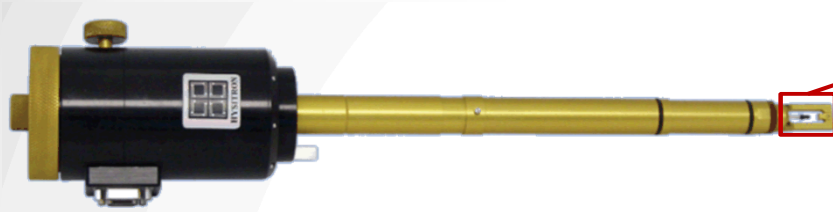
Hysitron PI95 In Situ Nanoindentation TEM Holder
