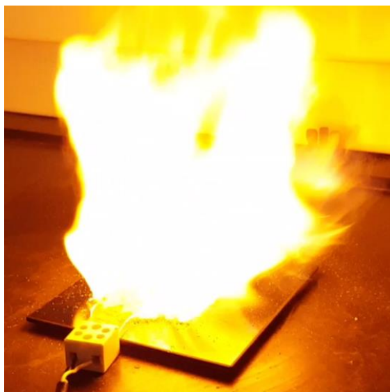
FIGURE 2. The Accelerated Combustion of a 4:1, by Mass, Mixture of Silver Nitrate and Cellulose
