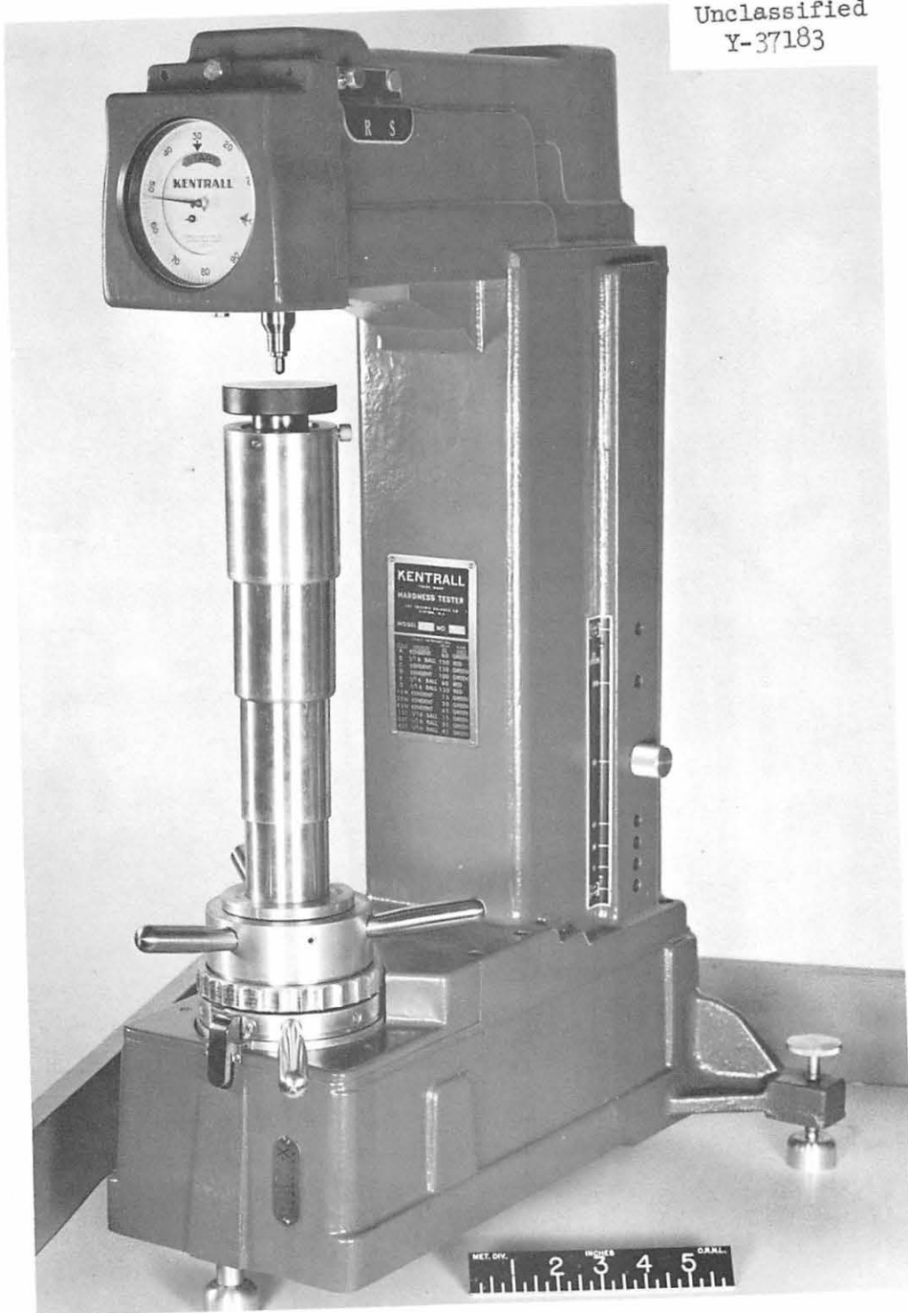
Fig. 26. Extended Range Hardness Tester for In-Cell Service.
