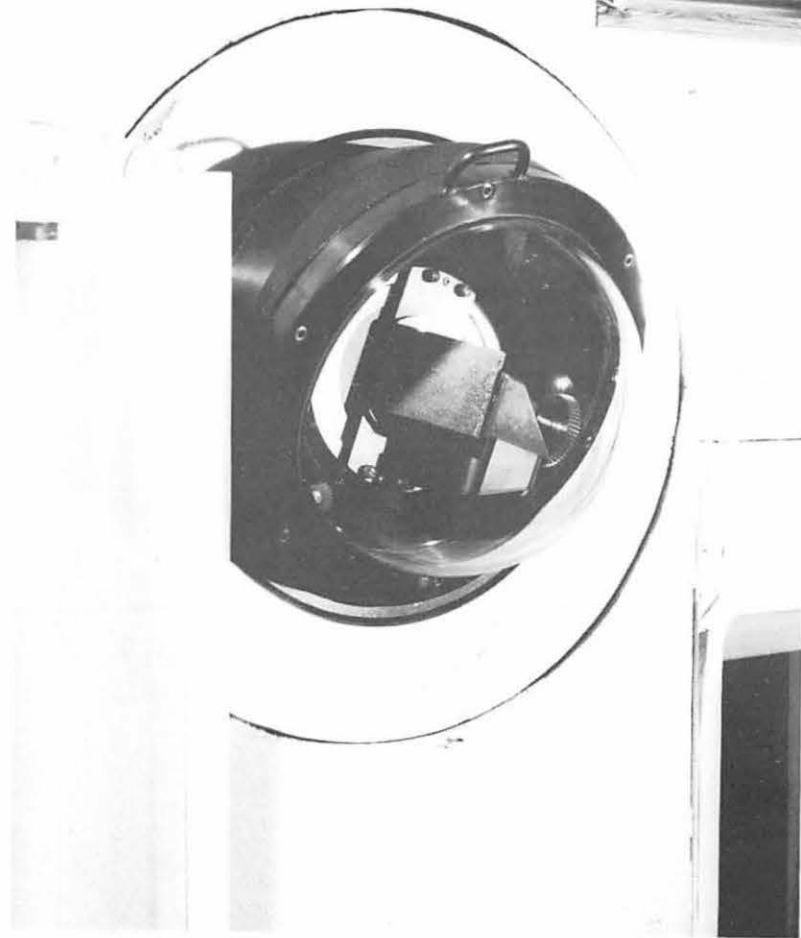
Fig. 10. In-Cell Appearance of Seal and Dome Features for Periscope.
