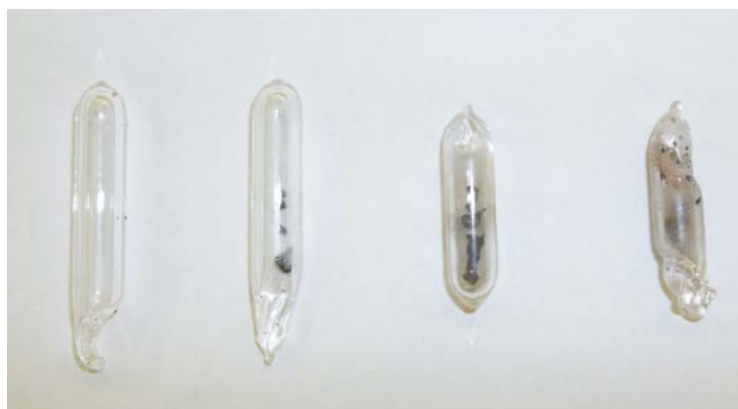
Figure 3. Photograph of sample ampoules. From left to right: no sample (empty), plutonium (not used in this irradiation), HEU, and NU.
