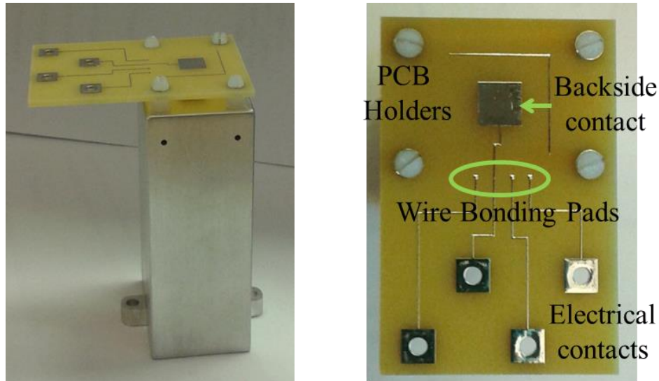
Figure 8: (Left) The aluminum Printed Circuit Board (PCB) holder mounts into the mass spectrometer and holds the PCB in the correct location. (Right) A top view of the PCB. The device will be adhered to the large pad at the top center of the PCB (forming a backside contact). Wire bonding will be used to make the remaining three electrical connections.
