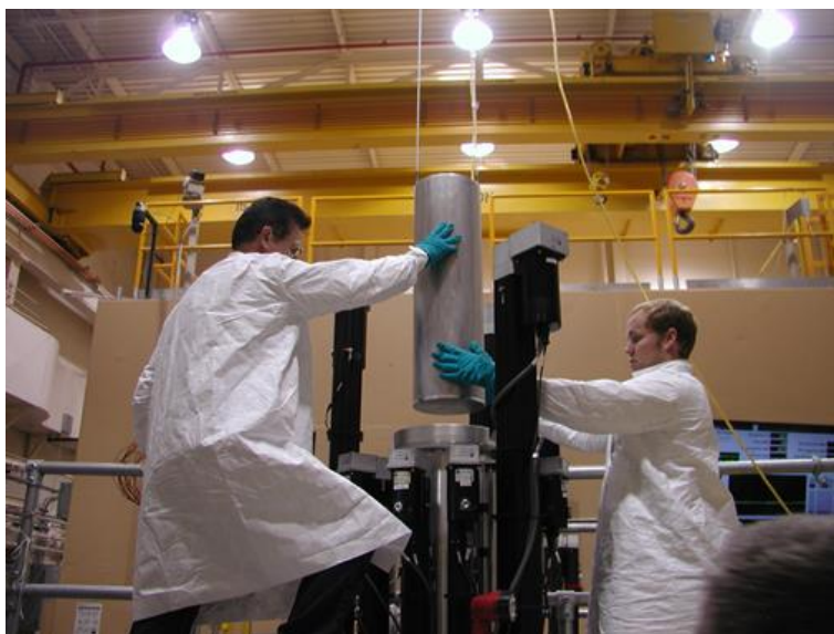
Figure 8. Installing the CdPoly Bucket into the ACRR Central Cavity.
