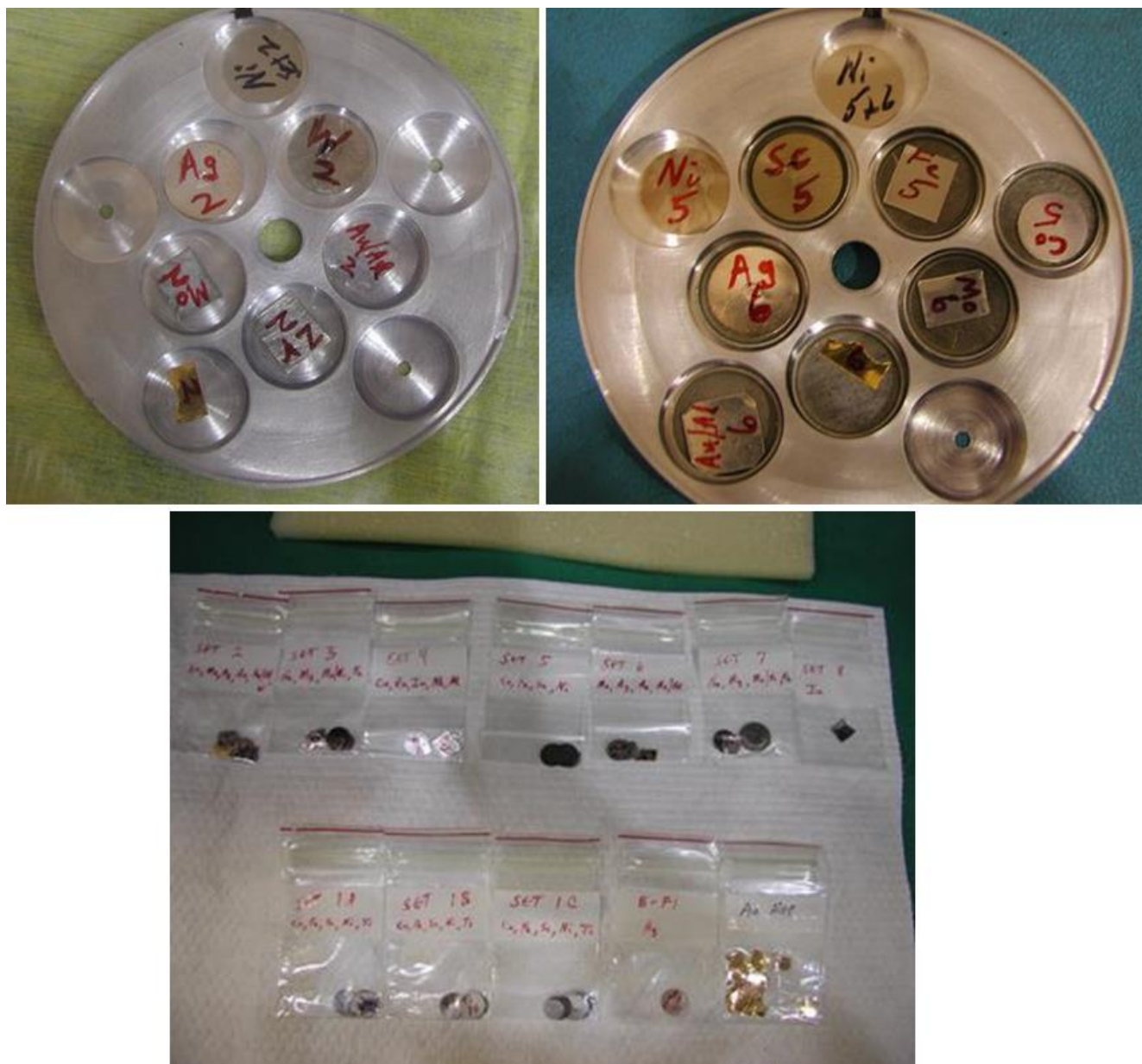
Figure 14. Aluminum Dosimetry Tray and Foil Packets Awaiting Irradiation.
