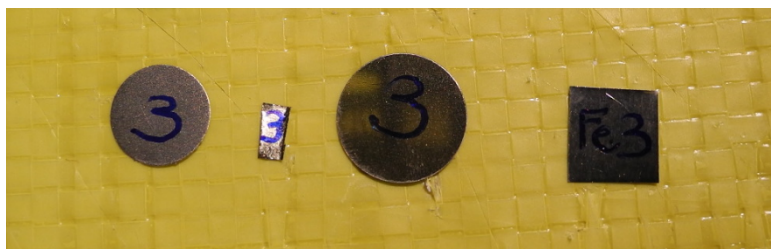
Figure 12. Typical Dosimetry Foils - Left to Right: Co, Sc, Ni, and Fe.
