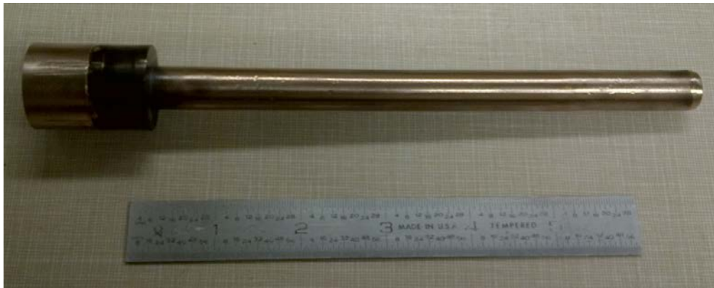
Figure 4- Photo showing the 026 extrusion with the die still attached.
