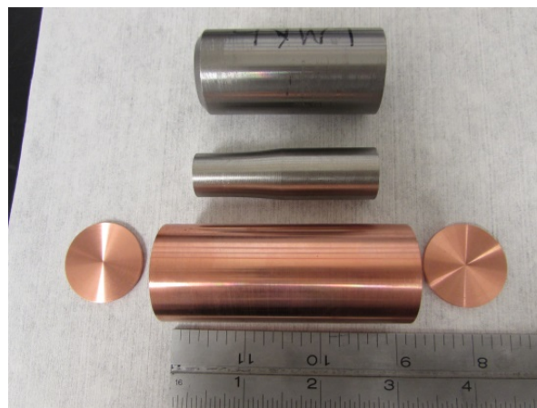
Figure 7 – 9YWT Billet with Machined Copper Tube and End Caps in Preparation for the First Stage Extrusion
