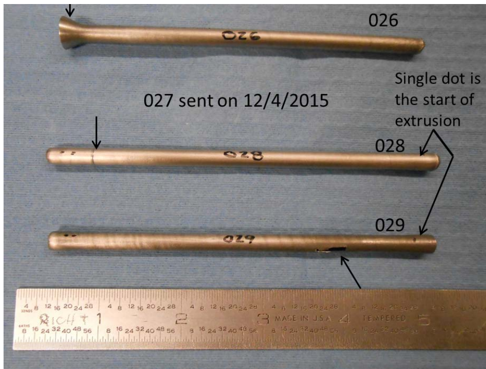
Figure 5 Photos showing hydrostatically extruded tubes after removal of billet cladding and mandrel materials.
