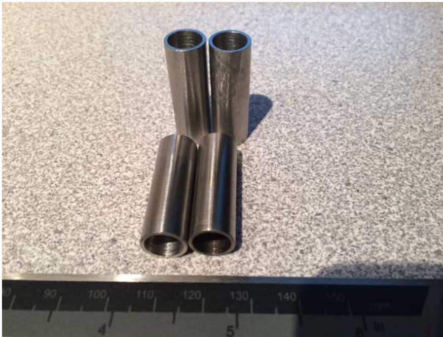
Figure 1- Photo showing original tubes of 14YWT sent to CWRU from LANL.
