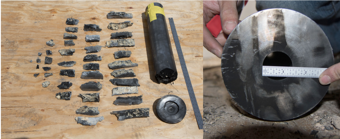
Figure 7. Tube fragmentation from the Baseline 2 test with full density PBX 9502 pellets (left). Tube distension from Baseline 3 test with pour density molding prills (right).
