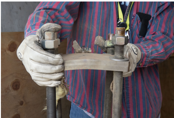
Figure 8. Endplate deformation (ignition-end) from the DDT 1 test with full density PBX 9502 pellets. Stronger endplates are recommended for future test versions.
