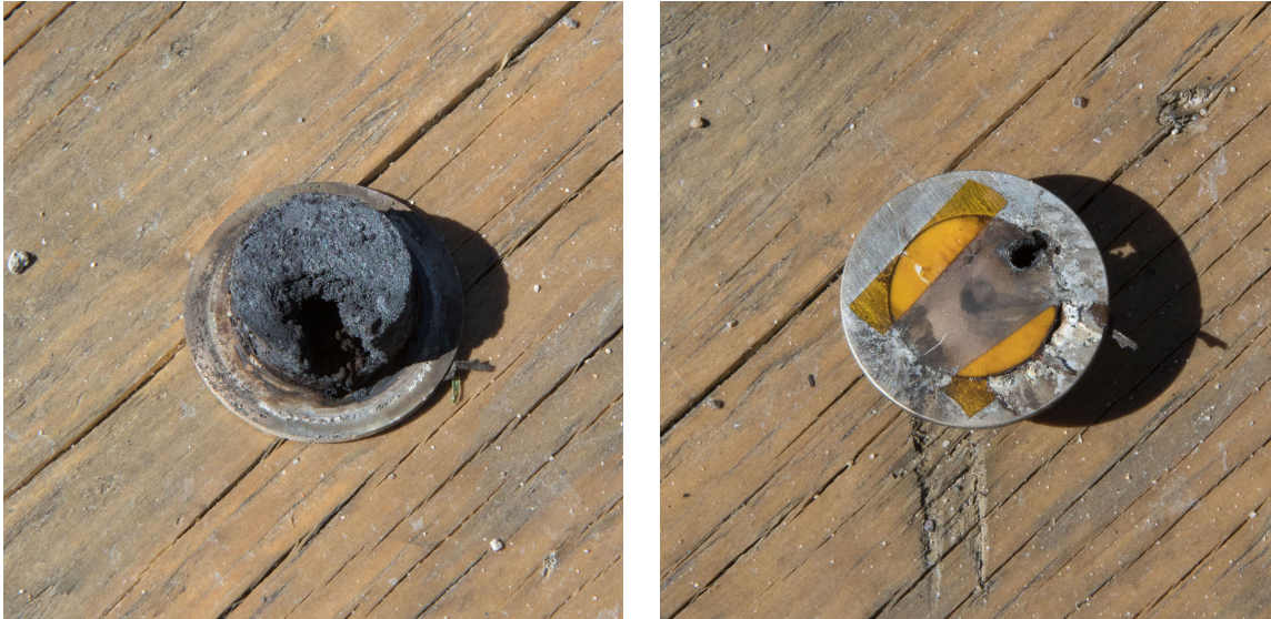
Figure 11. The IHE-side of the aluminum igniter cup with a gas channel eroded at the 6 o'clock position (left). The other side in the igniter cup assembly showing and eroded gas channel through the ceramic tamper at the 1 o'clock position (right).
