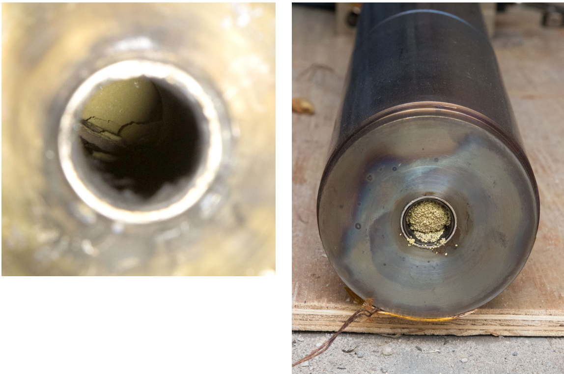
Figure 10. Compacted molding prills on the ignition end of the DDT 2 test (left). Un-compacted prills on the opposite end of the tube (right).
