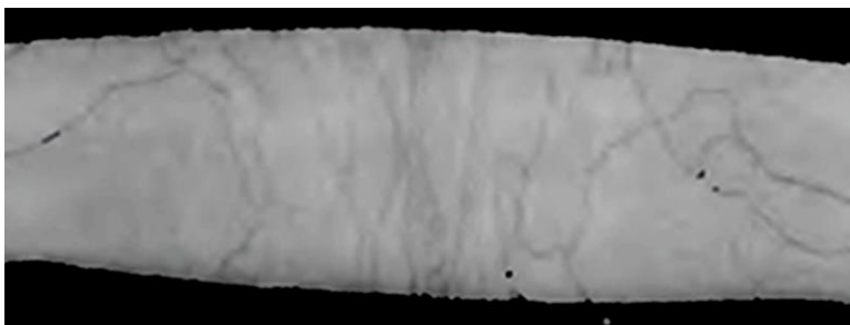
Figure 18: Photo of the weld center-line microstructure of a typical GTA weld in iridium. Note the essentially continuous single grain boundaries oriented vertically in the section. The weld was made at travel speed of 5 mm/s (12 ipm).
