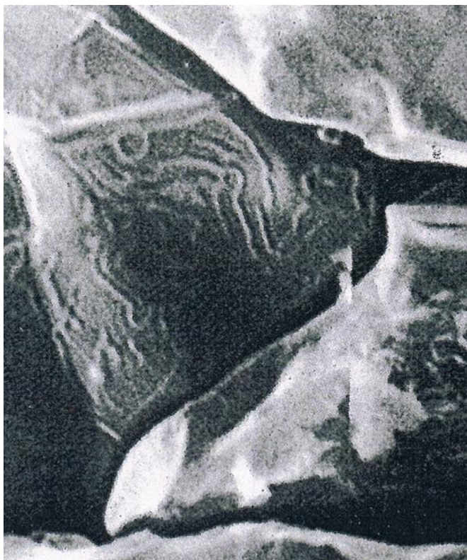
Figure 32: SEM picture of a crack face in the weld quench area in the DOP26-OP material showing the ridge structure indicative of eutectic formation on that grain facet, from [19].
