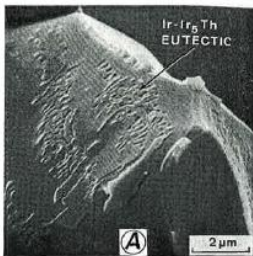
Figure 13: SEM picture of an arc weld fracture surface in DOP26-OP material showing the \text{Ir} + \text{Ir}_5\text{Th} eutectic (from [9]).
