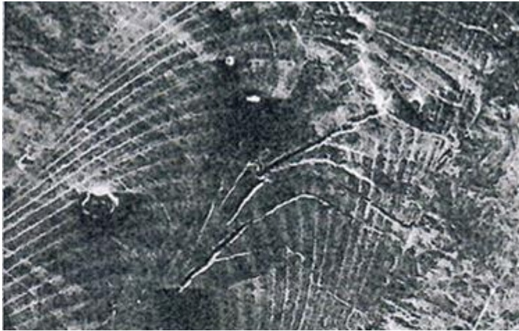
Figure 30: Picture of the inside surface of a typical weld showing the “weld quench” cracks.
