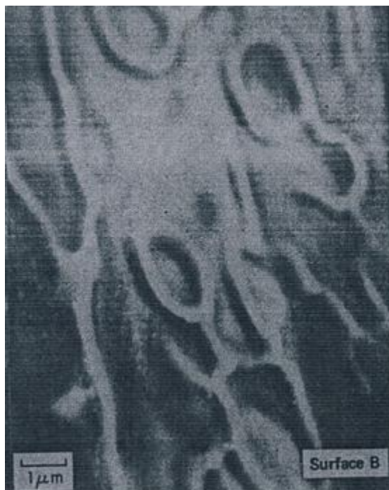
Figure 5: SEM picture of the fracture surface from a weld solidification crack in the DOP-26. The rounded features are grain boundary cavitation (gas) voids.
