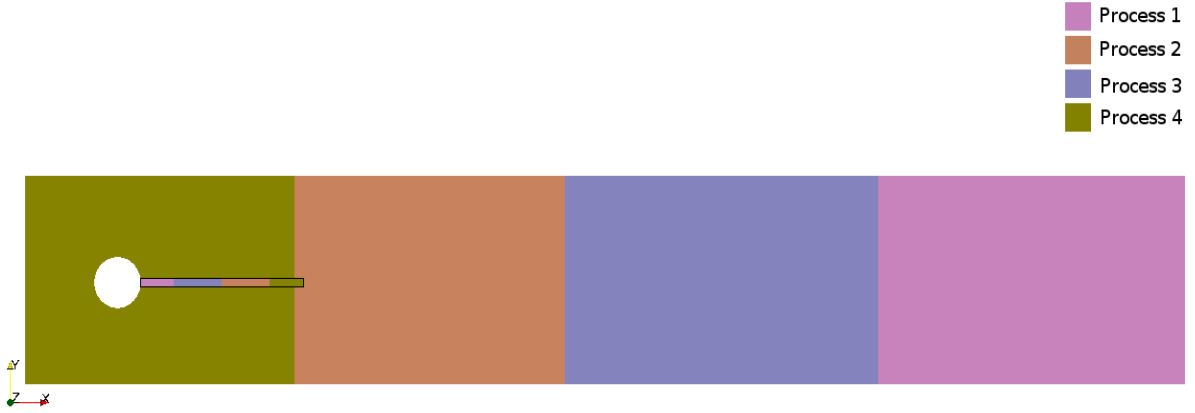
Figure 28: Partitioning of the simulation domain for parallel Heron Turek verification problem.
