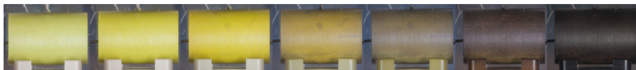
Figure 27. Selected stills from the time-lapse sequence of Test 2, showing evolution of discoloration of the sample. Total duration of this sequence is 38 minutes.
