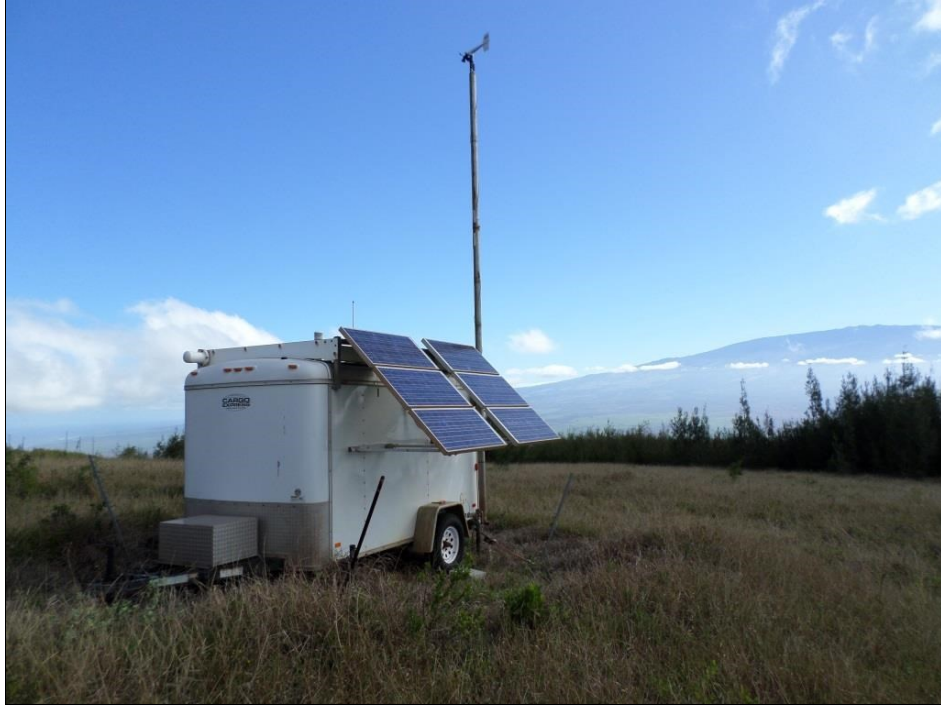
Figure A9.3.2: Self-powered, mobile Kaheawa Sodar on Maui.
