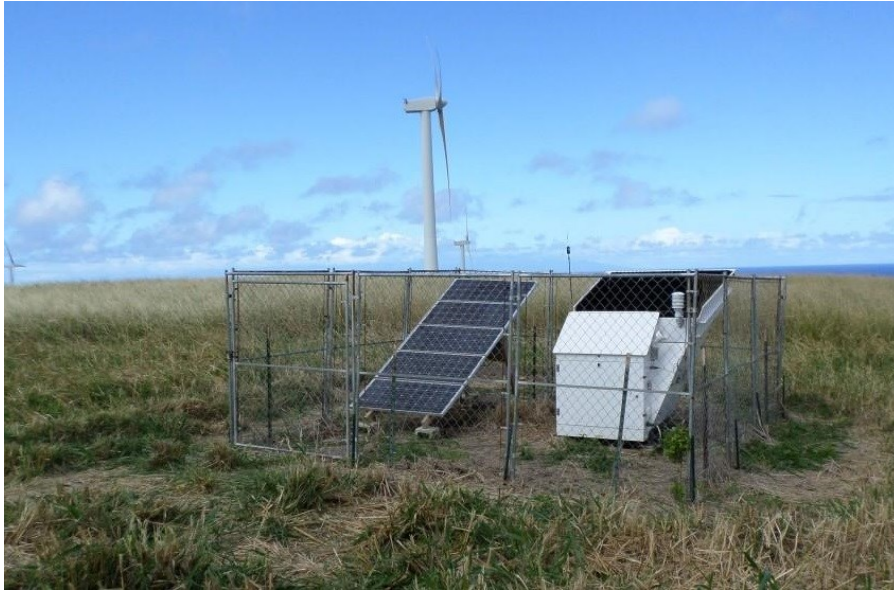
Figure A9.3.1a: Solar powered, battery back-up HRD Sodar on Big Island providing data for both HRD wind facility and Auwahi wind facility on Maui.
