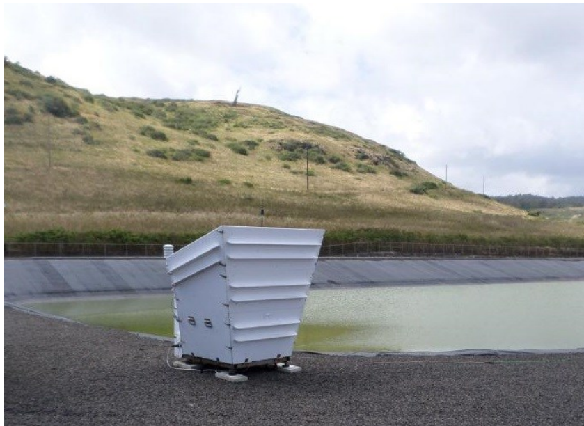
Figure A9.3.1b: Local powered, battery back-up Turtle Bay Sodar on Oahu providing data for Kahuku Wind Farm and SWIFT forecasting.
