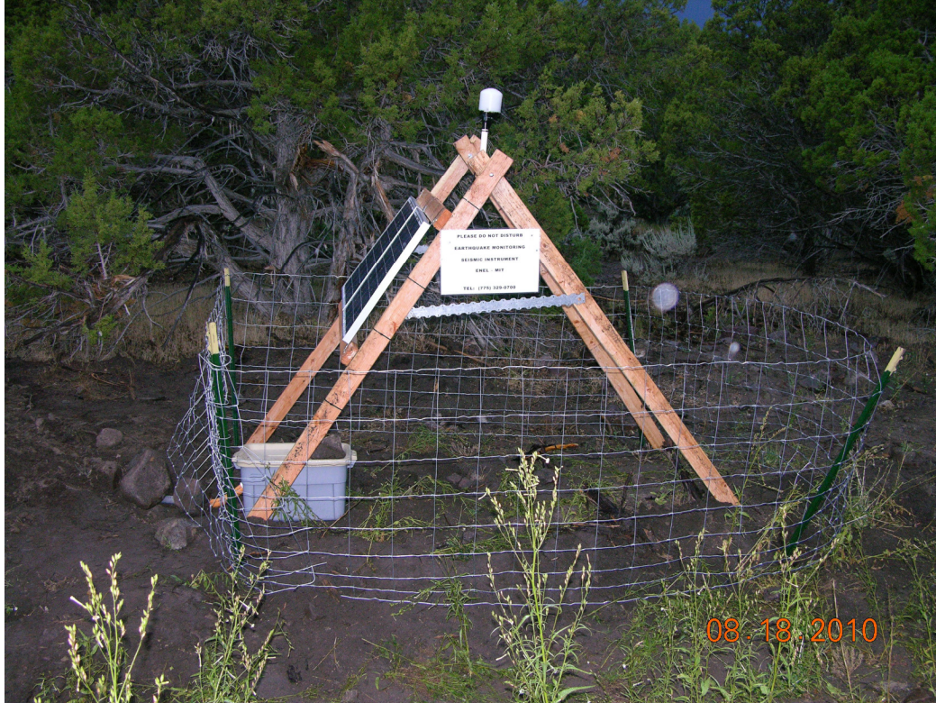
Figure 22. A typical seismic station installed for this project. Two solar panels are used for each station to charge the battery.
