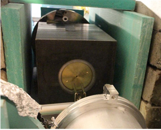
FIG. 2. The square steel collimator shell and brass inserts with 6 mm aperture located at approx. 30 m, looking upstream. Borated polyethylene and concrete block shielding surround the steel plates.
