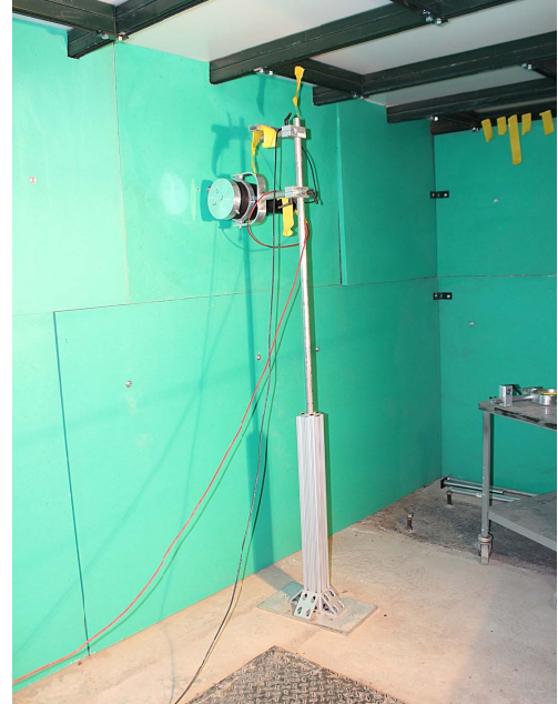
FIG. 3. Li-glass detector mounted at 65 m in FP-13.
