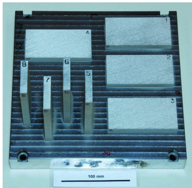
Figure 2 : Optical photograph of EOS builds on 304L SS baseplate
