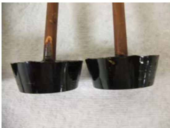
Figure 4a. New epoxy samples after exposure to ethanol at 120°C for 1 year
