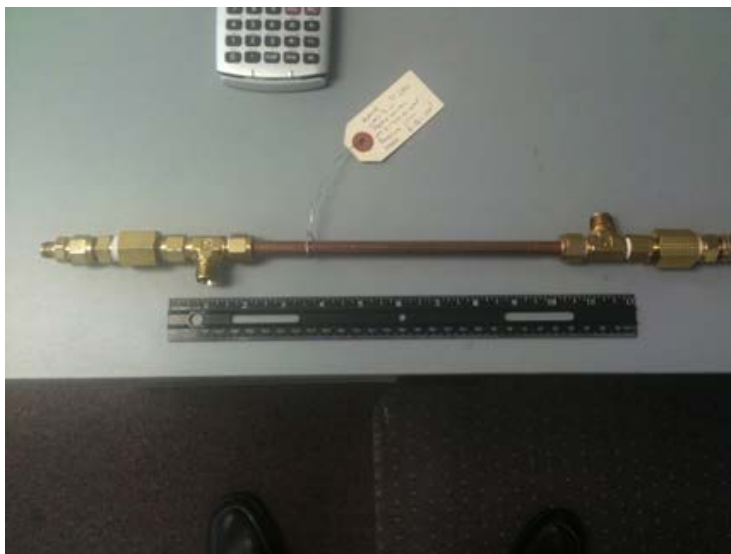
Figure 9. Hollow fiber membrane minimodule made for qualifying batch of membrane made for ethanol dehydration.
